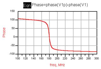
Here we see the result of the frequency sweep. The peak loop gain occurs at 179 MHz as does the 0 degree phase shift point. The oscillator should start up at this frequency. Note that the loop gain is rather low for reliable startup. The tapped capacitor impedance transformer should be revised for higher small signal loop gain.
