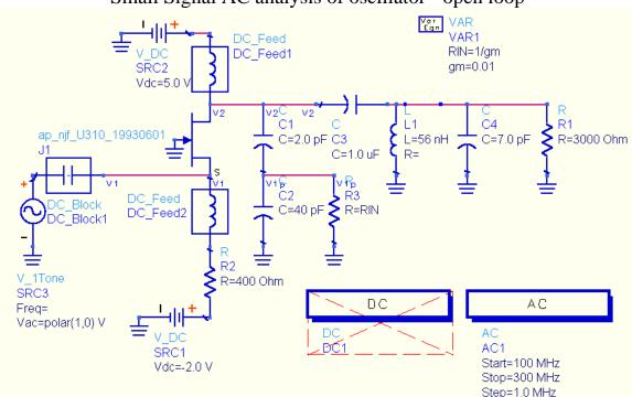
Small Signal AC analysis of oscillator - open loop
