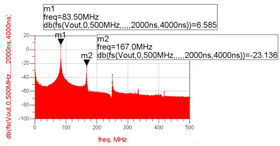
Output spectrum from a transient analysis simulation. The fft (fs function) is used to display frequency spectra. The format of the function is:
