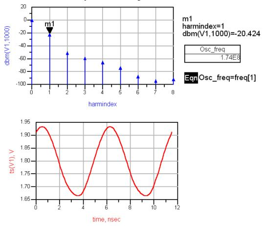
The output from a HB oscillator simulation can be either a frequency spectrum or a time domain representation of any voltage or current in the circuit. You can see that the
