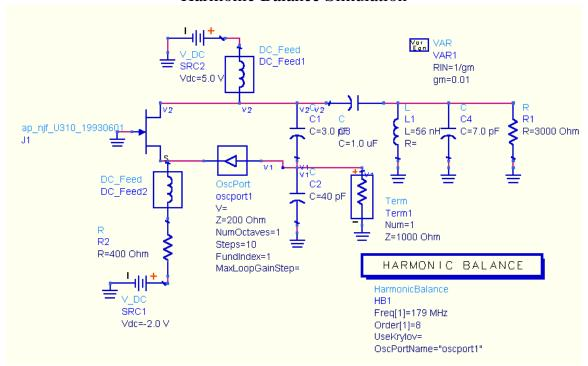
Harmonic balance simulation can also be used for closed-loop oscillator analysis. HB has be advantage that it calculates the steady-state solution directly and is relatively fast compared with transient analysis (when it converges). To simulate an oscillator, the ADS OscPort must be inserted into the signal path. The arrow must point in the right direction.
