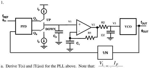
a. Derive T(s) and  $|T(j\omega)|$  for the PLL above. Note that:  $\frac{1}{\Delta \phi} = \frac{1}{2\pi C_F}$
