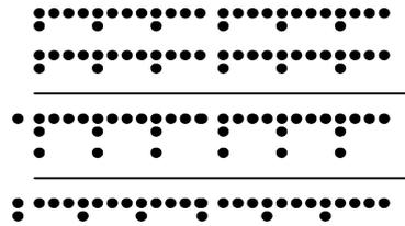
Figure 1. Reduction of the addition result to a 2-deep result.
