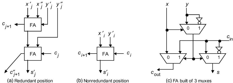
Figure 2. Adder cells for representations of Table 2, and a 3-multiplexer full-adder.
