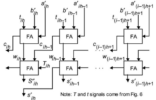
Figure 8. Representationally closed adder for SDB hybrid-redundant numbers.
