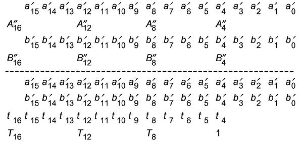
Figure 5. Symbolic representation of step 1 in adding two SDB hybrid-redundant numbers.
