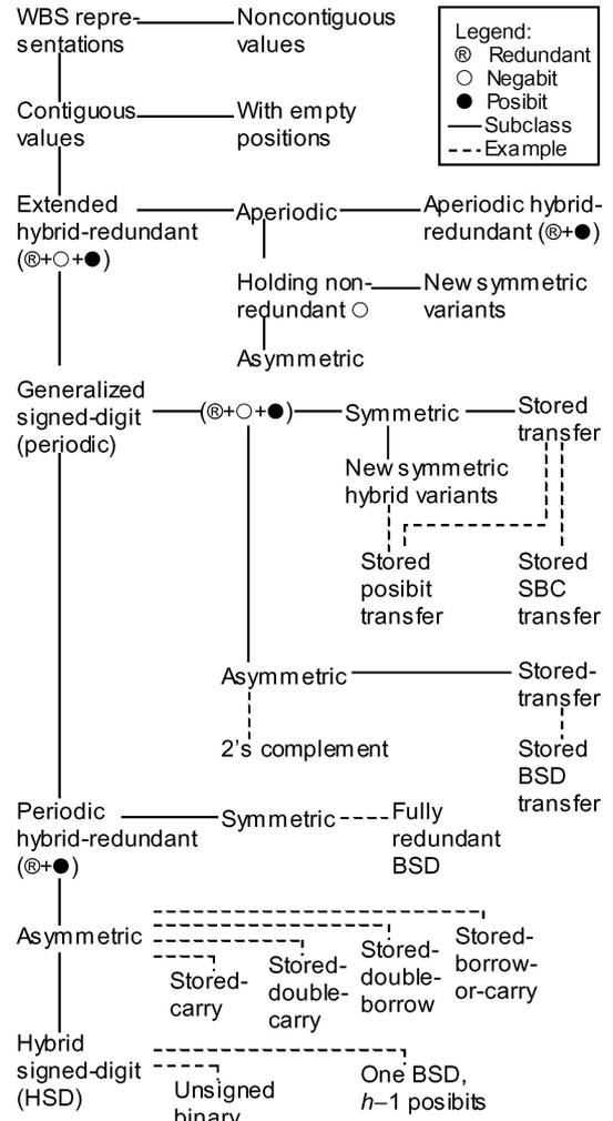
Figure 3 The hierarchy of number representations using weighted components (tree branches go from left to right and top to bottom).
