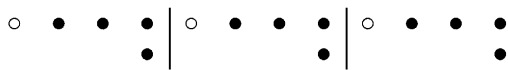
Fig. 13. A canonical WBS encoding of an extended hybrid-redundant number system with the symmetric digit set [-8,8] .
