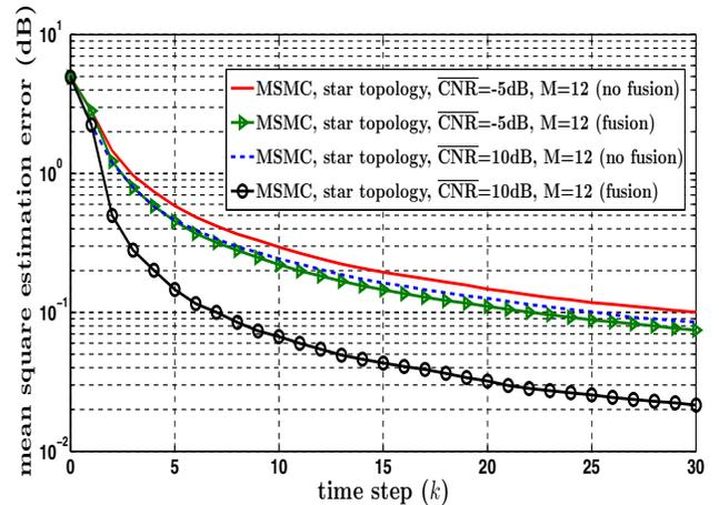
Fig. 4. Impact of fusion on the performance of MSMC over a star-shaped graph.
