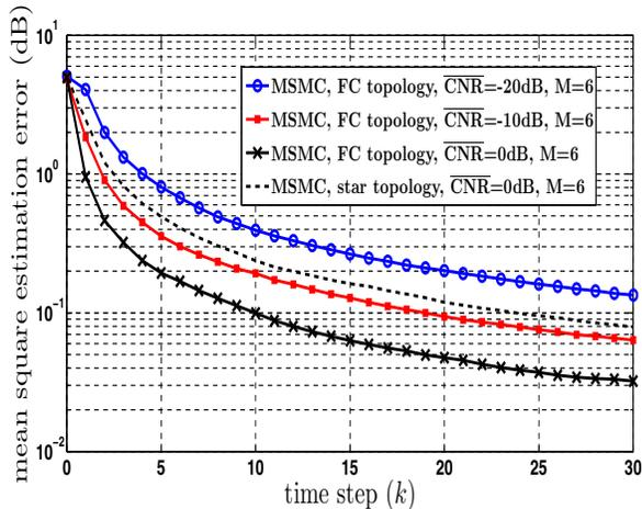
Fig. 3. Performance of MSMC for the case of no fusion over both a fully connected and a star-shaped graph for different link qualities.
