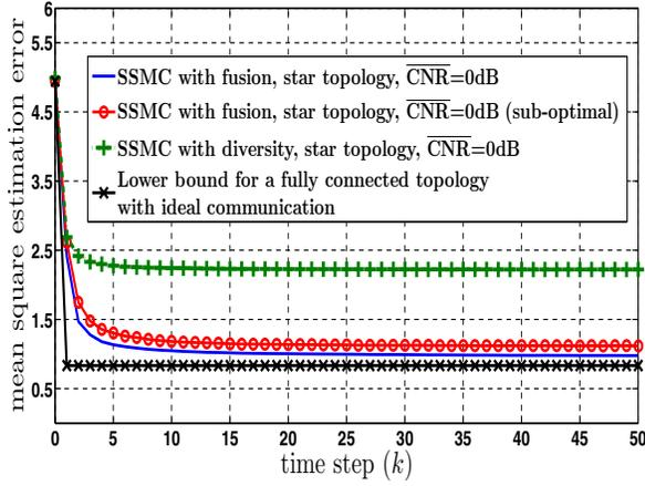
Fig. 1. A comparison of fusion and diversity techniques for the SSMC case with  $M=6$ , the graph is star-shaped with fading channels for non-ideal communication cases.
