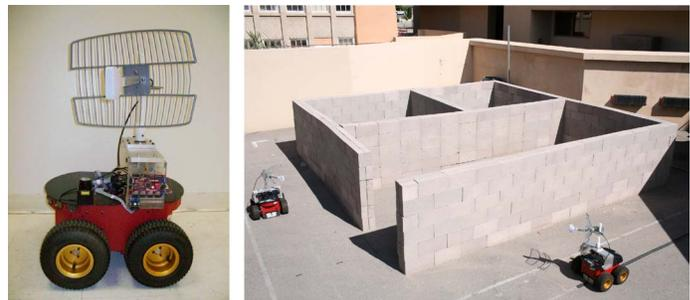
Fig. 11. (left) A Pioneer P3-AT robot equipped with our servo control mechanism/fixture, adaptive narrow-beam directional antenna and Hokuyo laser scanner; (right) two robots using laser scanners and wireless measurements in order to map an obstacle structure that includes occluded parts.
