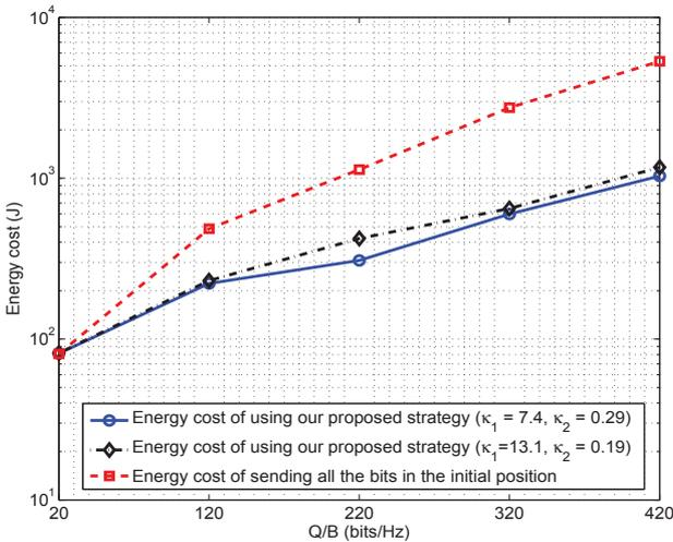
Fig. 2. Performance of our strategy as compared with the case where the robot sends all its data at its initial position. It can be seen that the robot can benefit more from motion as the number of bits increases.
