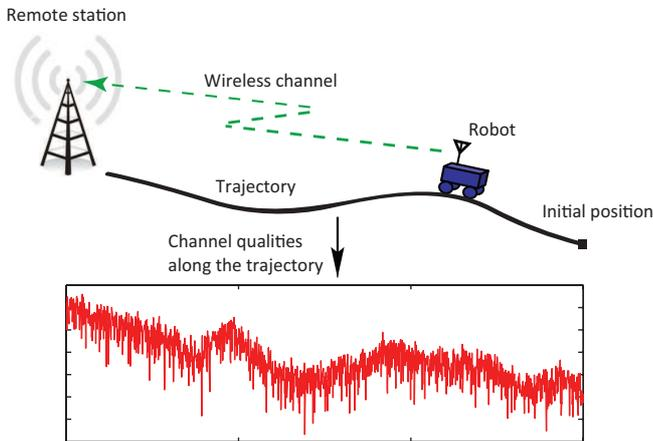
Fig. 1. The robot needs to transmit a number of given bits to the remote station, under a given time budget and BER constraint. It is allowed to move along a predefined trajectory to find a position where the channel quality is high. The goal of the robot is to minimize its total energy cost, including both communication and motion energy costs.
