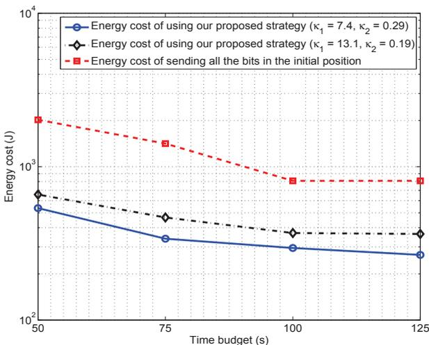
Fig. 3. Performance of our strategy as compared with the case where the robot sends all its data at its initial position. It can be seen that the robot can benefit from motion significantly.
