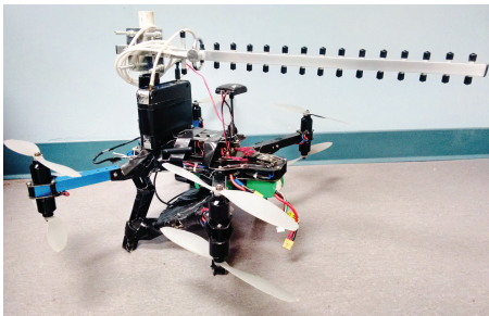
Figure 8: A 3DR X8 octo-copter used in our experiments.
