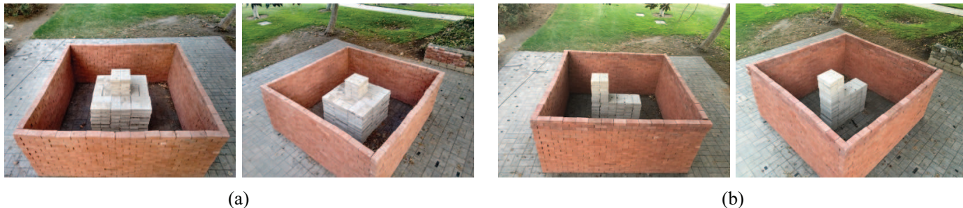
Figure 9: The two areas of interest for 3D through-wall imaging. (a) shows the two-cube scenario and (b) shows the L-shape scenario. For better clarity, two views are shown for each area.
