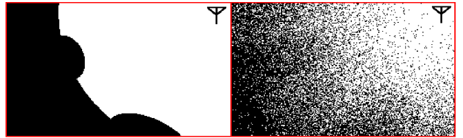
Fig. 6. Examples of a binary channel (white areas indicate that channel quality is above a threshold) – (left) channel generated based on knowing the positions of the obstacles and considering only large-scale fading and path loss and (right) the same channel after adding Rician-distributed fading.
