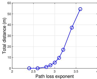
**Fig. 3.** Average total distance traveled as a function of path loss exponent ( $n_{PL}$ ) for the known channel case.
