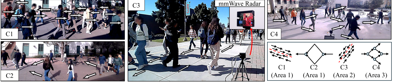
Figure 3: Experimental setup: A mmWave MIMO radar transmits FMCW pulses, which reflect off of individuals moving in a crowd according to the white arrows, emulating the configurations C1-C4 in three different areas. The inset shows a front-facing view of the radar. See color PDF for best viewing.
