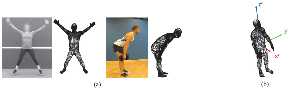
Fig. 2. (a) Sample reconstructed 3D human mesh from a snapshot of (left) a person doing jumping jacks and (right) a person doing stiff-leg deadlifts. (b) The Local Coordinate System (LCS), defined with respect to the human body.
