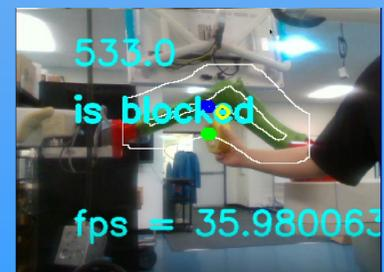
Our program can detect objects around the outer layer of the robotic arm. When the program identifies the objects that could cause collision, it sends a 'blocked' signal. To raise the performance of collision avoidance, our camera tracks the center of arm, indicated by the yellow circle in the center of robotic arm
