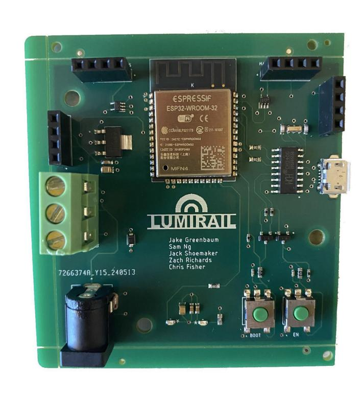
Our custom PCB incorporates an ESP-WROOM-32-N4 microcontroller enabling Wi-Fi & Bluetooth connectivity, ensuring seamless interaction with the Android application and internet. It enables control of the individually addressable PL9283 LEDs and the MAX7219 LED dot matrix, and other electronic components to complete our final product.
