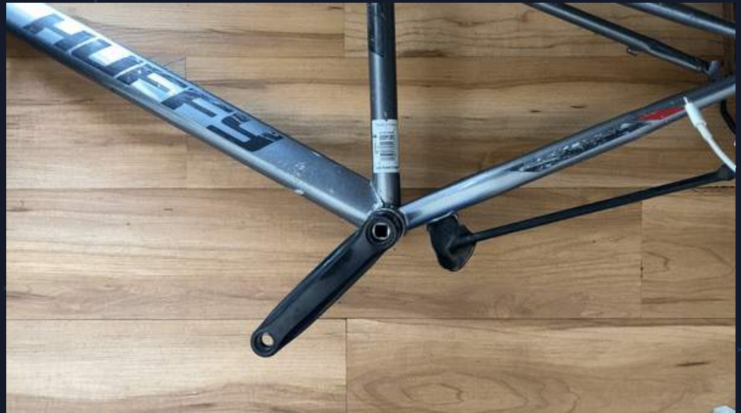
Figure 1.7. Secure the crank arm with a bolt
