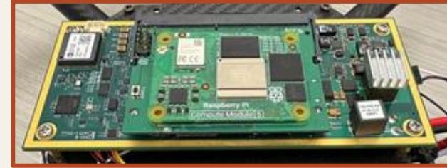
CM5 mounted on Varmint using Pi in the Sky Carrier Board
