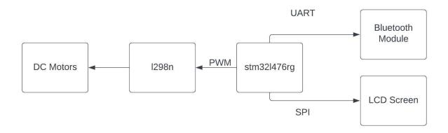
Parts: L298n DC motor controller HC-SR04 Ultrasonic Distance Sensor HC-05 Bluetooth Module ILI9341 TFT LCD
