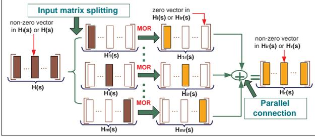
Fig. 1. The BDSM model reduction scheme for a linear network with  $m$  input ports, which is based on column-by-column moment matching. After input matrix splitting, the original model is decomposed into  $m$  MIMO subsystems. Then using the projection process,  $H_{ir}(s)$  captures the first  $l$  moments of  $H(s)$ 's  $i$ -th column. Finally, the parallel connection of all ROMs guarantees the preservation of  $H(s)$ 's first  $l$  moments.
