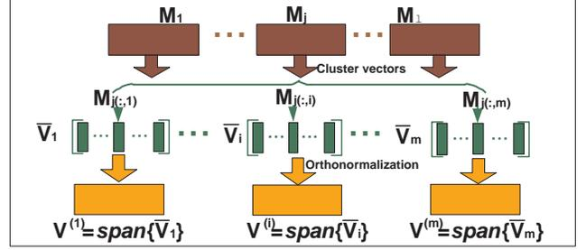
Fig. 2. Projection matrix construction in BDSM. In this figure,  $M_j = ((s_0 C - G)^{-1} C)^{j-1} (s_0 C - G)^{-1} B$ ,  $j = 1, \dots, l$ . The  $i$ -th columns of  $M_j$ 's are grouped to form  $\bar{V}_i$  ( $i = 1, \dots, m$ ). And then  $V_i$  is computed such that  $V_i = \bar{V}_i$ , for  $i = 1, \dots, m$ . Note that, in PRIMA the projection matrix for (1) is constructed without clustering, such that  $V = \text{span}\{M_1, \dots, M_l\}$  with more computational cost.
